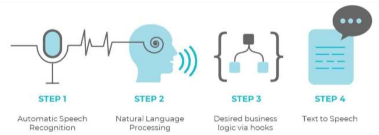
Fig.1. Diagram depicting how a voice based virtual assistant work
